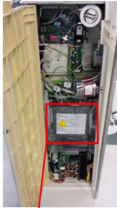
Plastic cover in front of mass-flowmeter (IB 1426100)
